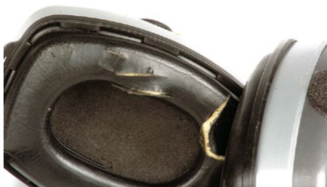
Figure 36 Damaged earmuff seal
