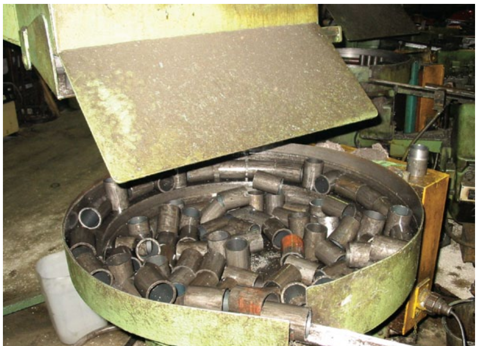
Figure 8 Lining of a bowl feeder with rubber for reduced impact noise
