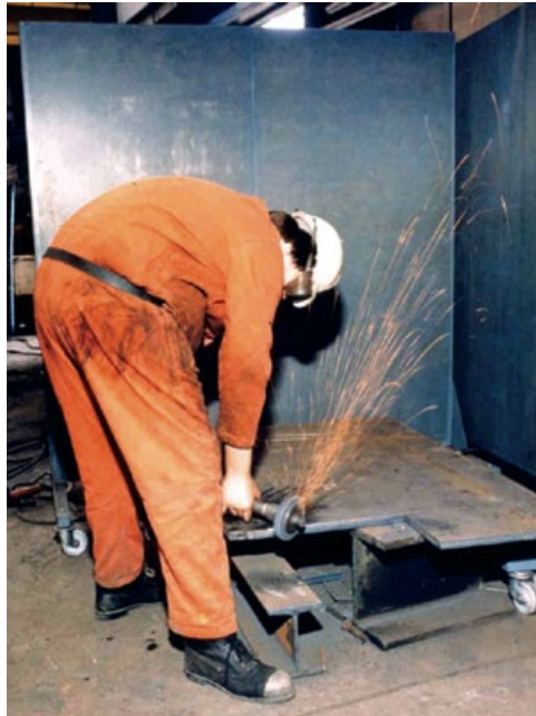
Figure 10 Moveable acoustic screen in an engineering workshop
