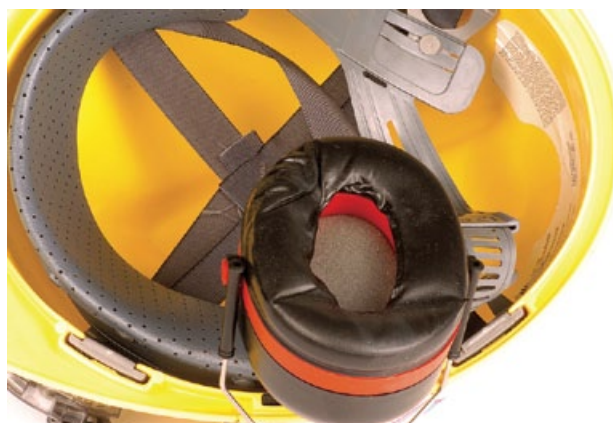
Figure 37 Damaged helmet-mounted earmuff seal due to prolonged storage in 'up' position
